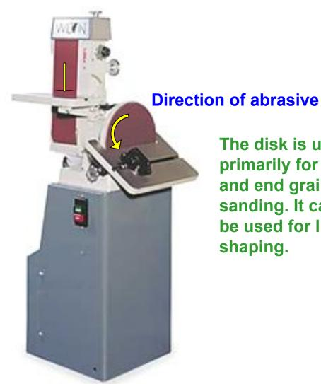
The disk is used primarily for rough
