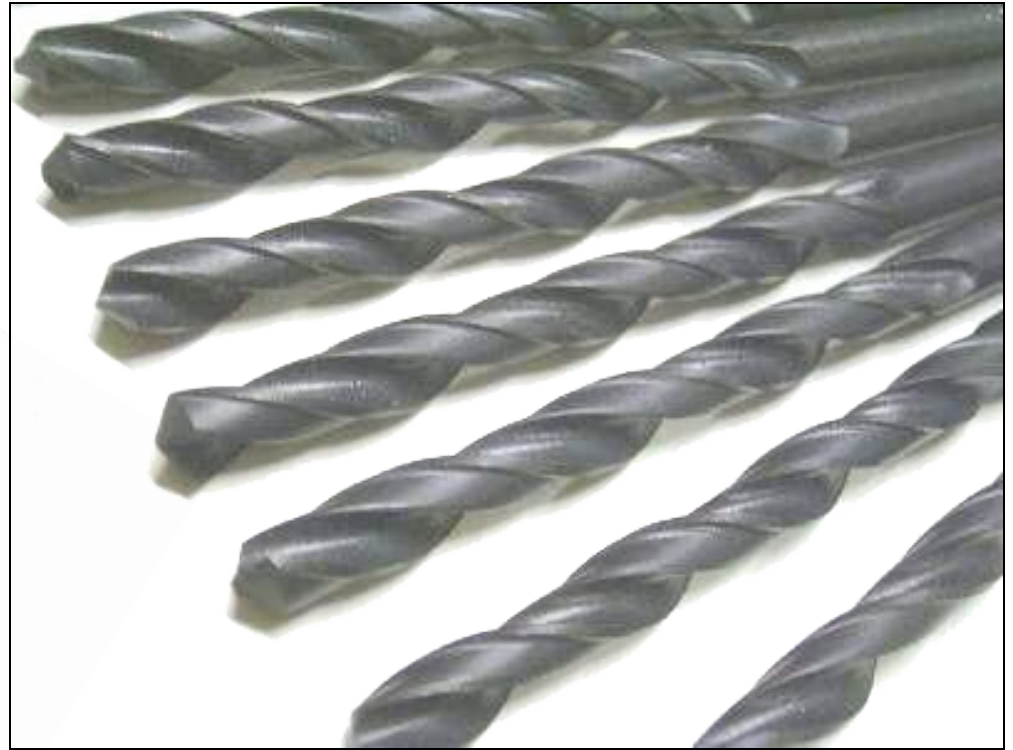
Use twist drills for drilling smaller holes.
